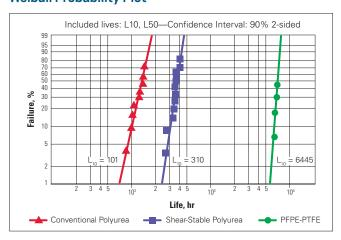
Still skeptical, the reliability superintendent asked to run an ROF test to compare Krytox AUT 2E45 to comparable offerings that were available. The results of the test demonstrated that Krytox lubricants were more effective and lasted from 21 to 64 times longer than competitive lubricants. After seeing the data, the reliability superintendent and his team were ready to implement a Krytox lubricants "lubed-for life" solution at the mill.
