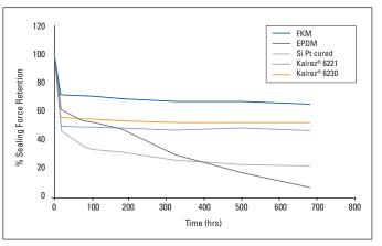
ISO 3384 method B, 140 °C air, sealing force retention %.
