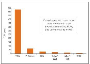
EPA method 415; TOC tests performed on 1" sanitary seals, immersed in 50 mL of sterile WFI at 100 °C/24 hr. The solution was then diluted to 100 mL and analyzed.
