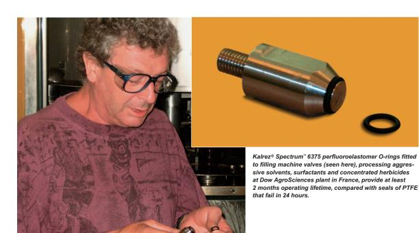
By switching from O-rings of PTFE to DuPont Performance Elastomers Kalrez® Spectrum® 6375 perfluoroelastomer parts at its plant in Drusenheim, France, Dow AgroSciences S.A. has seen seal lifetime increase from an average of one day to two months, leading to greater availability of its filling machines, major improvements in safety and reliability, reduced maintenance, and cost savings, reports Michel Blondel, mechanical maintenance leader at the plant (seen here).
