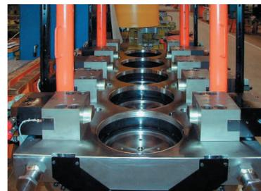
Hilma-Römheld GmbH, of Hilchenbach, Germany, a leading manufacturer of heavy duty clamping systems for metals, plastics and rubber processing, has switched to DuPont Performance Elastomers Kalrez<sup>®</sup> Spectrum<sup>™</sup> 7075 perfluoroelastomer parts to seal its hydraulic clamp range, with the goals of ensuring long-term resistance to highly aggressive Oemeta HF/DU hydraulic fluids at 250°C, saving costs, and increasing the reliability of the system.
