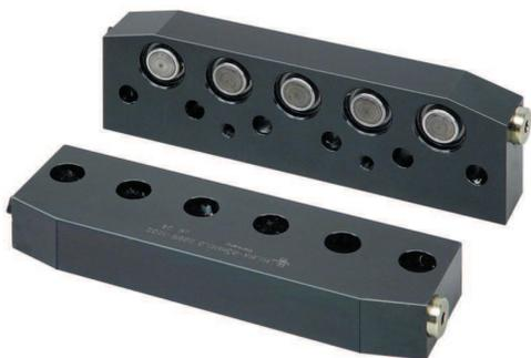
*Clamping bar on Hilma-Römheld heavy duty clamping system, equipped with Kalrez<sup>®</sup> Spectrum<sup>™</sup> 7075 perfluoroelastomer O-rings resists pressures up to 400 bar, temperatures as high as 250°C, and handles clamp forces of 25-1250 kN without leakage of hydraulic fluid.*
