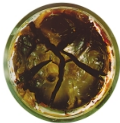
In oven at 232 °C (448 °F) for 40 hr: Hydrocarbon—40% wt loss
