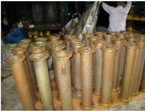
Pump column sections
