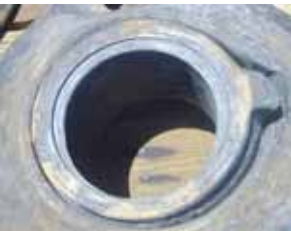
Metal impregnated graphite 3.5 year service 0.5" (12.7mm) Wear, shaft damage Not serviceable
