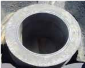
Vespel® CR-6100 3.5 year service 0.02" (0.51mm) Wear, no shaft damage Serviceable
